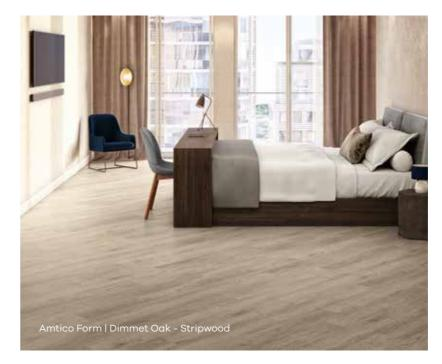
Amtico's state-of-the-art sound reduction technology helps reduce noise pollution by up to 19dB by using an integrated 1mm closed-cell PVC foam. Not only does it increase comfort underfoot but it can also be used in high-traffic areas such as schools, offices and public service spaces.
